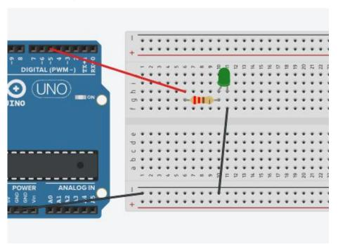
Move your positive voltage to pin 5 on the Arduino and open the following file and run it:
